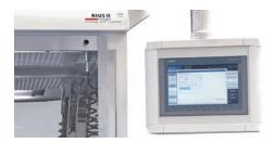
12" BASIC TOUCHPANEL with intuitively operable software. Simple operating due to password-secured user-levels and the possibility to save test processes. Continuous monitoring of safety relevant functions. Optional comfort touch panel with separate keyboard with easy to clean glass surface available.
