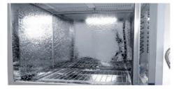
ANALYSIS AREA (approx. 1200 x 800 x 800) with polished stainless steel interior. For components up to 100 kg. Automatic cleaning of all four walls and fast achievement of blank values due to integrated wall flushing device.
