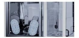
DOUBLE WORKING SPACE: Two analysis areas with polished stainless steel interior for different part geometries. Very small components in the millimetre range up to parts weighing 100 kg. Basin 1: 800 x 800 x 800 mm. Basin 2: 300 mm half round basin with ultra sound.
