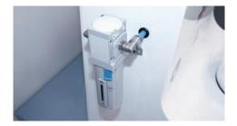
EASY MAINTENANCE and reduction of excessive moisture by a slightly emptiable collecting container.
