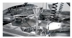
ANALYSIS BASIN (600 x 750 mm) with polished stainless steel interior. For components up to 15 kg. Smallest parts with high requirements can be tested with optional funnel. Extraction in the front work area.
