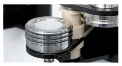
THE USER-FRIENDLY, lifting and tilting membrane holder includes three individual cascade rings with tweezer leads for safe and simple membrane fitting and removal of 0 47 mm membrane filters.
